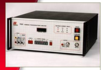
uildline Model 7620 is a very wide band transconductance amplifier. By connecting the output from a stable voltage source to the 7620, it is capable of producing outputs up to 20 amps over a specified frequency range of DC to 100 kHz, and a usable frequency range extending to 1 MHz.
